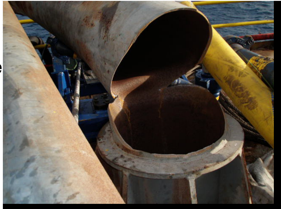
Failed Starboard King Post
