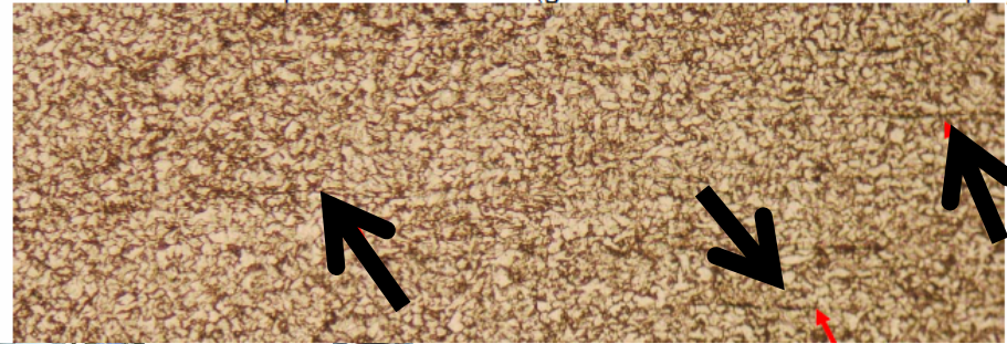
Microstructure of deck plate at location 1B (grains refined due to weld heat input).
