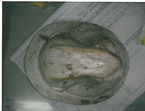
Photo 3 damage to Hard Hat
