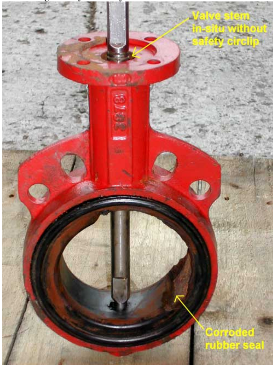
The damaged Bray Butterfly Valve
