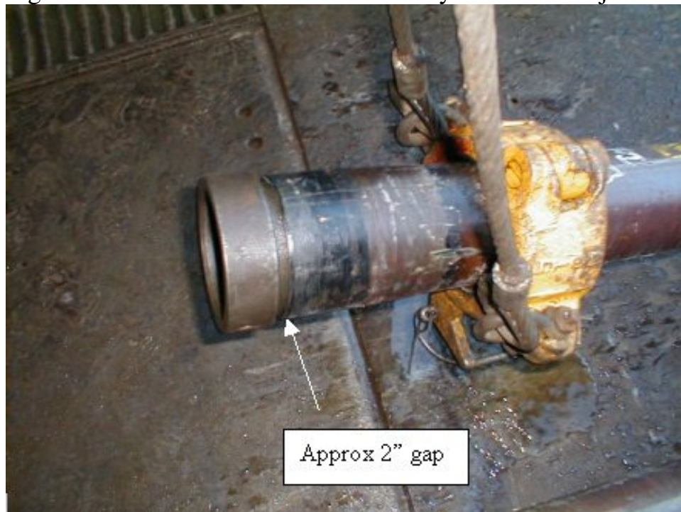
Figure A - Picture shows nubbin correctly screwed into joint
