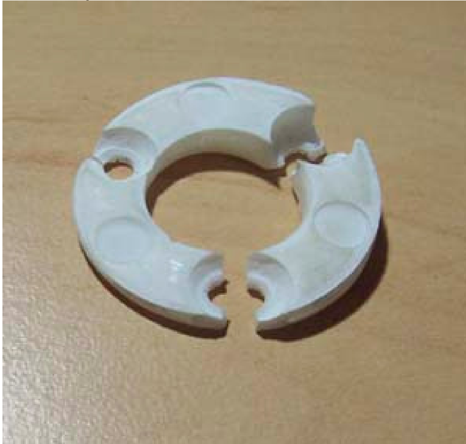
Broken Stop Pad
