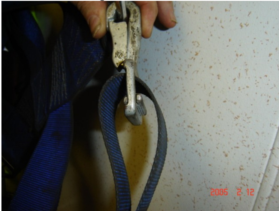
Incorrect buckle arrangement
