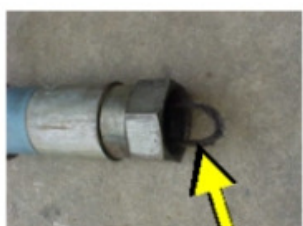
Some hoses have internal whip-check protection – wire rope up the inside of the pipe.
