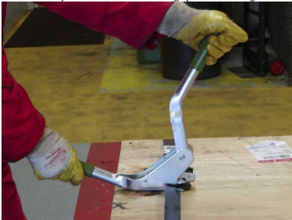
New tool keeps hands well clear and grips the banding
