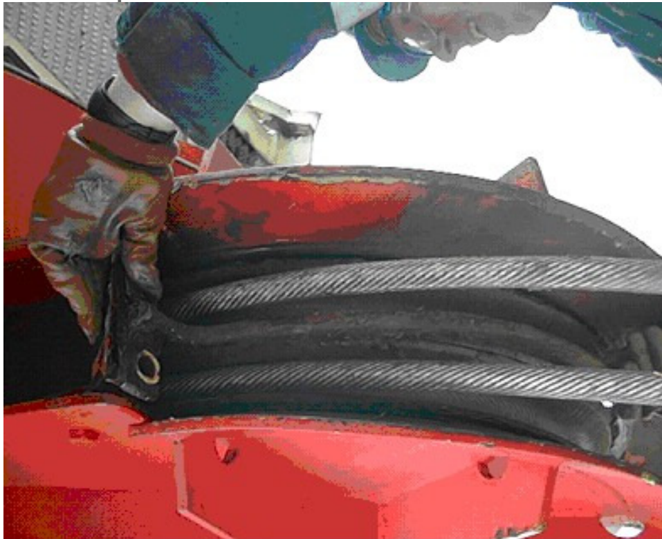
Bracket in place on sheaves
