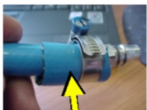
An example of an airline being used by a contractor. A piece of extra hose was fitted under the worm drive clip to allow the hose to be tightened onto the barbed air fitting.
