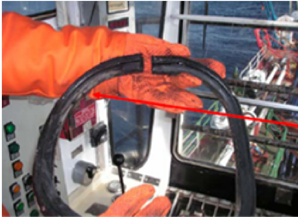
Picture of perished rubber window seal
