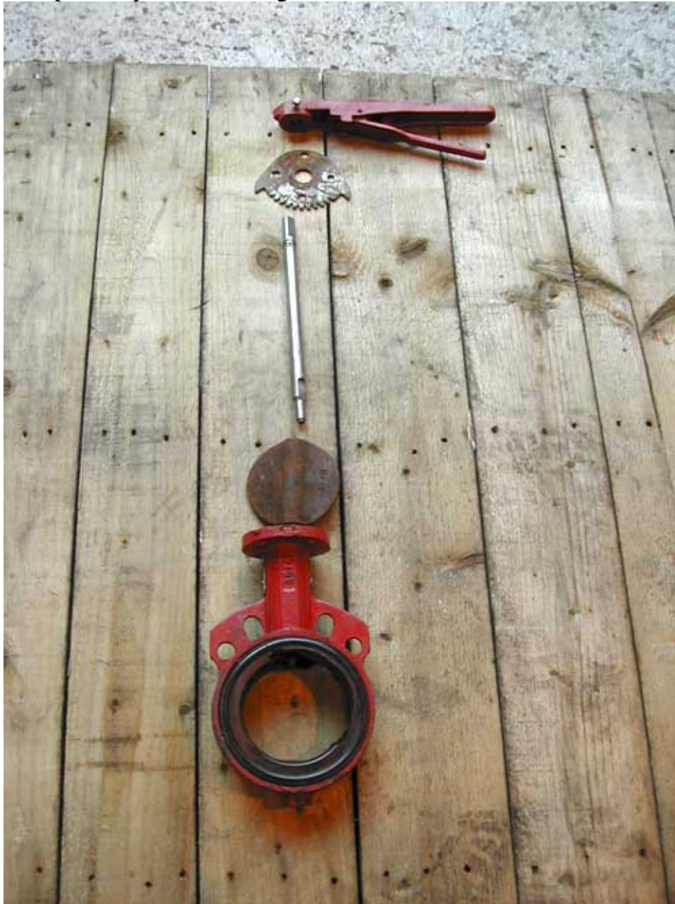
Component parts of damaged valve
