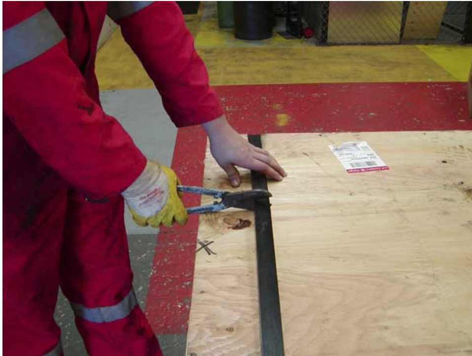
New tool keeps hands well clear and grips the banding
