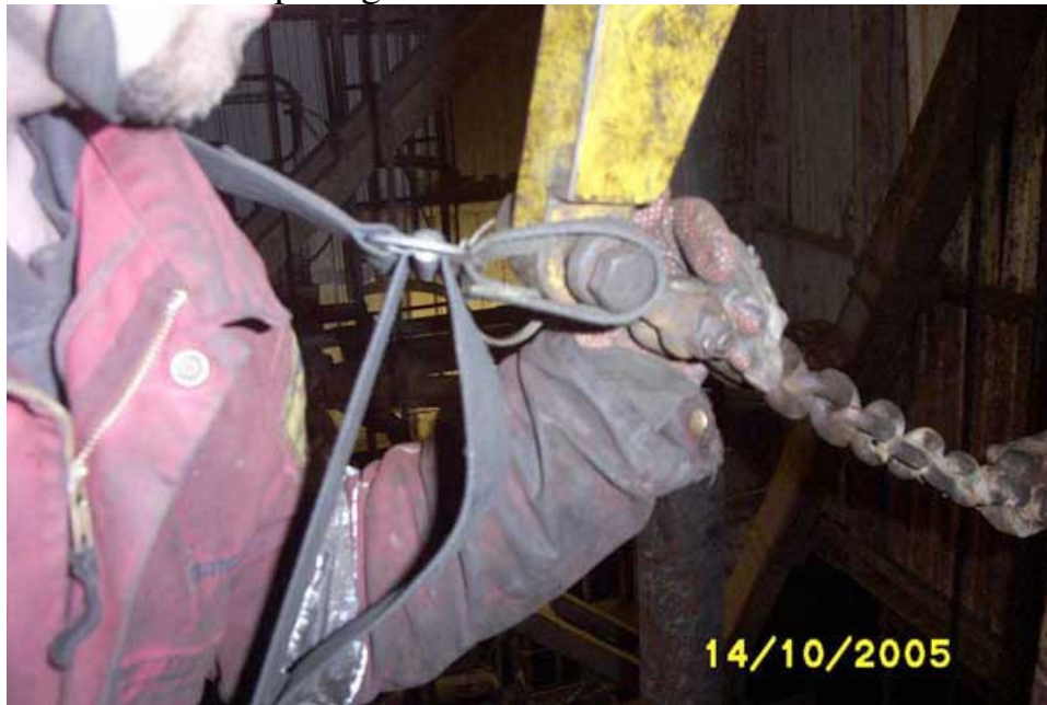
Linktilt with loop caught on nut
