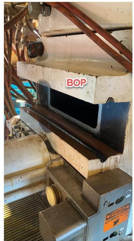
Picture 2: BOP Body Where Door Separated
