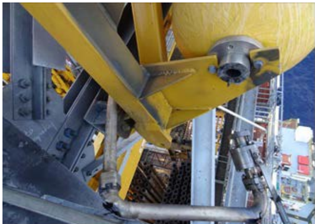
Failed CAPV and Interconnected Pipe
