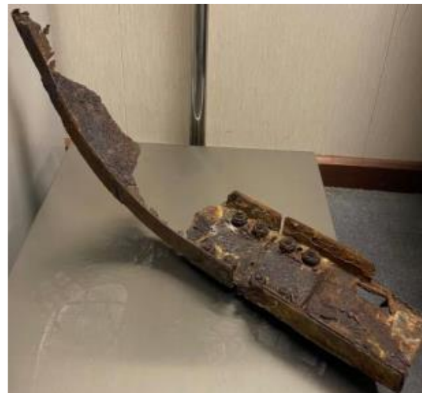
Potential dropped Object: – Piece of ladder rack weighing 3kg
