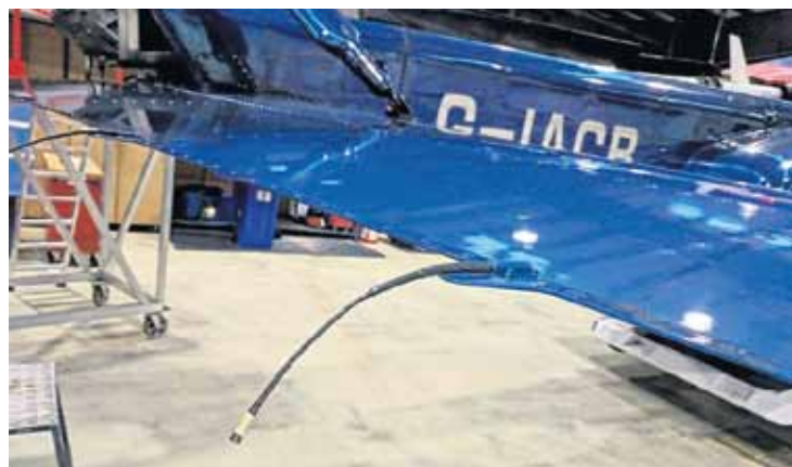
Cables on the helicopter allow static potential to equalise
